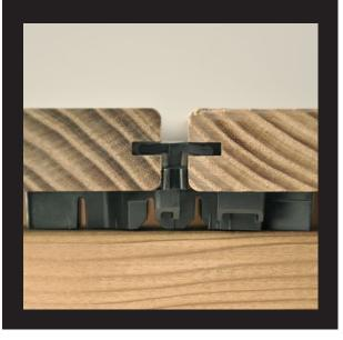
OVERVIEW Length 74mm | Width 66mm | Height 10mm Dimensions: joint spacing 6,3 mm POM polyoxymethylene black UV and weather resistant Material: UNIA System screw: hardened stainless steel or A4 Stainless steel Concealed Sliding point fixation Fastening type: Dimensionally stable and modified Decking profile: wood species with side grooved profiled decking boards
