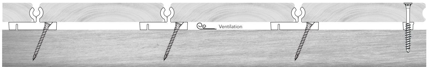
Partially visible screw connection for end and start boards
